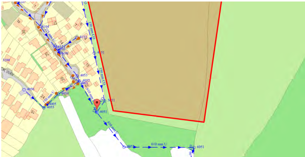
Figure 2: Surface water point of connection
