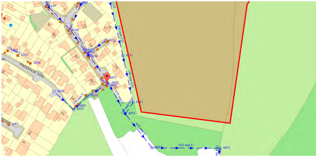
Figure 1: Your used water point of connection
